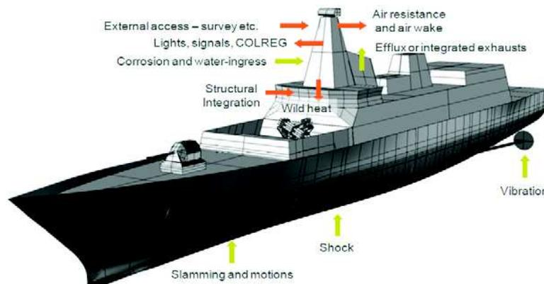
Figure 13. Issues of Concern for Naval Mast Design (Savage & Kimber, 2010).
