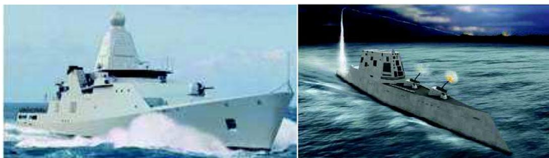
Figure 16. Typical Enclosed Mast on left ([www.thalesgroup.com](http://www.thalesgroup.com)) and enclosed mast as deckhouse (Hackett, 2011).
