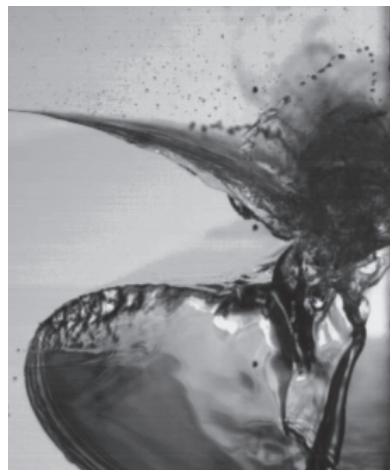
Figure 10: Free surface instabilities generated before a wave impact in a flume (Sloshel JIP)
