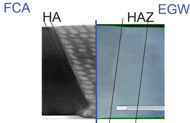
Figure 3: Weld Macros illustrating differing Heat Affected Zones for different welding processes.
