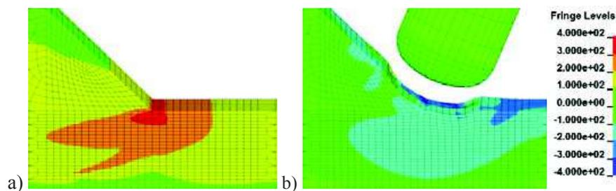
Figure 1: Transverse residual stress distributions and plastic deformation at weld toe; (a) as-weld, (b) after UIT.
