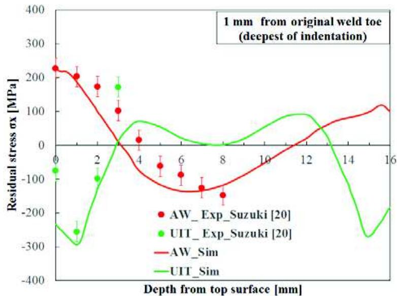
Figure 2: Distribution of transverse residual stress of as-weld and UIT specimens in the depth direction, and comparison with experimental results (Suzuki, et al., 2014).
