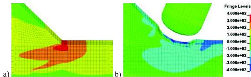
Figure 1: Transverse residual stress distributions and plastic deformation at weld toe; (a) as-weld, (b) after UIT.
