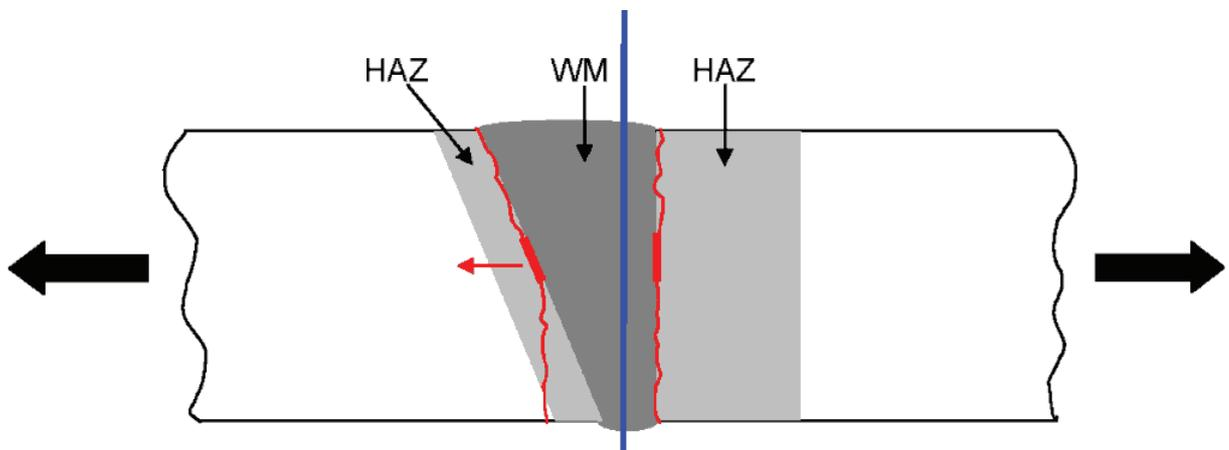
Figure 4: Likely Crack Paths depending on weld preparation detail.
