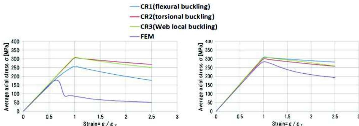
Figure 4 Comparison of CSR and FEM in stress-average strain relationships of stiffened panel
