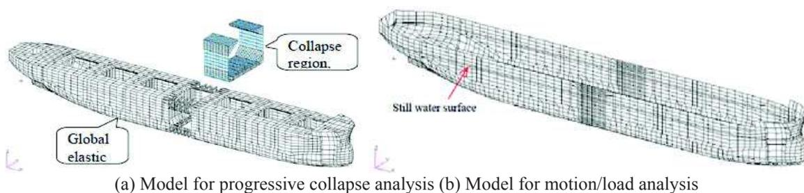
Figure 1.4 Two models for total system analysis [4].
