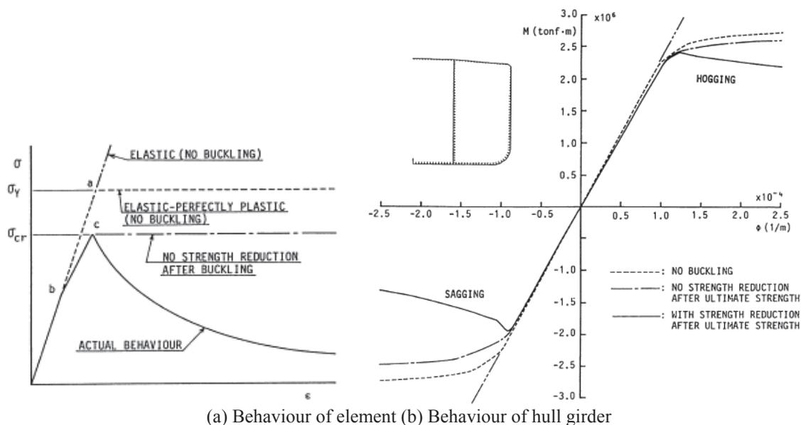
Figure 1.3 Influence of Element behaviour on global behaviour (by Smith’s method) [3].
