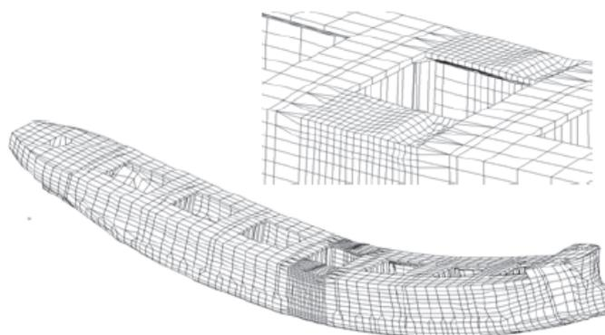
Figure 1.7 Sagging collapse mode in homogeneous loading condition [6].
