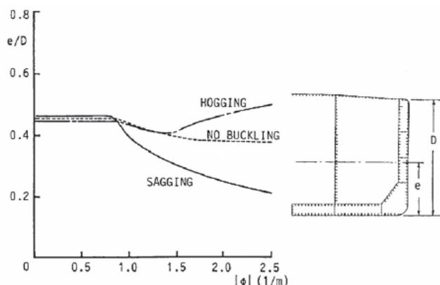
(b) Shift of neutral axis in cross-section
