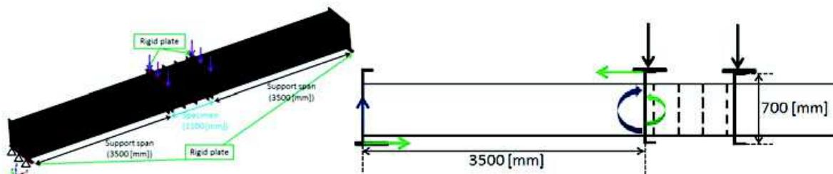
Figure 2 The schematic view for explanation of added bending moment induced by friction forces.
