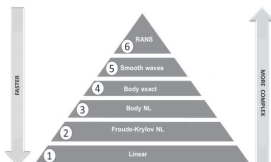
Figure 1. Level of idealisation for forward speed hydrodynamic solutions. Numbers 1 to 6 refer to levels 1 to 6 of idealisation according to Hirdaris et al. (2014a).
