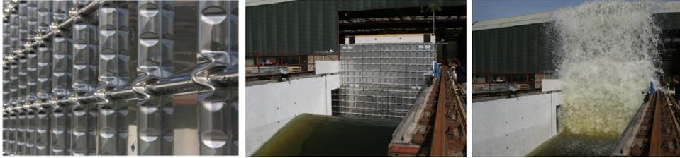
Figure 7: Quasi full scale impact experiments (Sloshel project)
