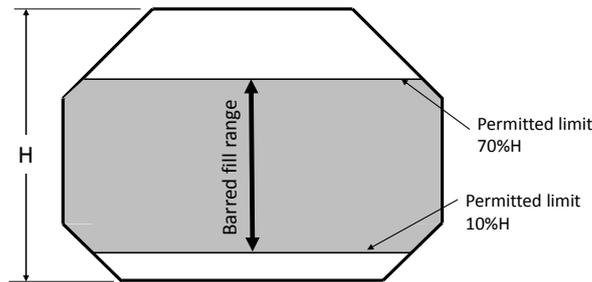
Figure 9: Membrane tank typical fill range limitation (GTT)
