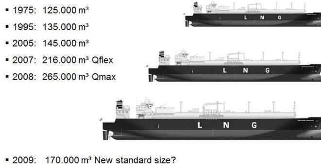
Figure 2: The development of standard LNG ship size
