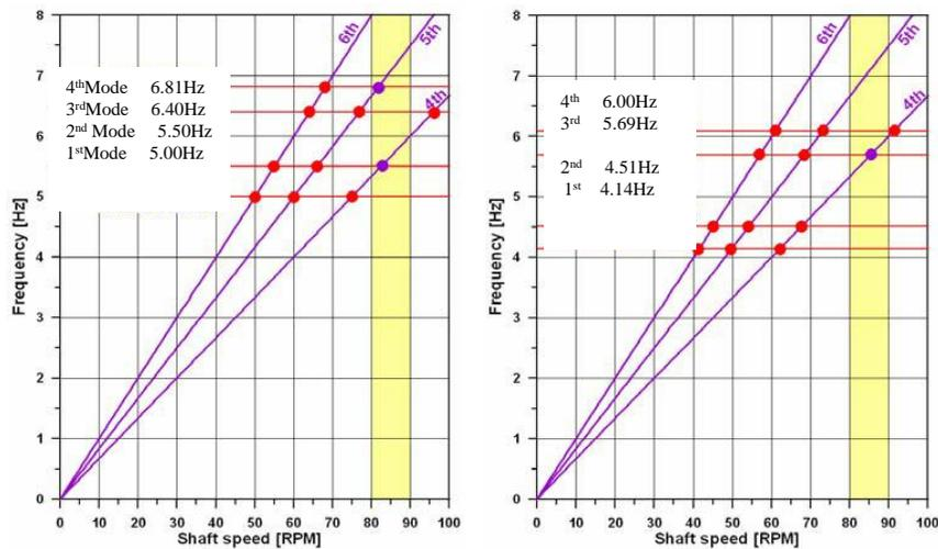
Figure 16: Campbell diagram for pump tower for empty (left) and fully filling (right) in membrane type (Lee *et al.*, 2006)
