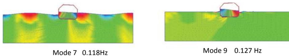
Figure 12: Natural vibration modes of the integrated fluid-structure interaction system (Xiong *et al.*, 2007a)
