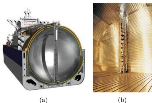
Figure 13: Pump tower within (a) Moss and (b) membrane types of LNG tanks ([http://expflow.com/lng\\_carrier](http://expflow.com/lng_carrier) and Lee, 2006, respectively)
