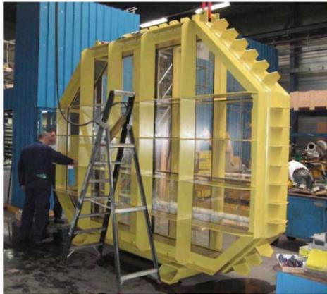
Figure 14: Overview Large scale (1:10) LNG Containment system model.
