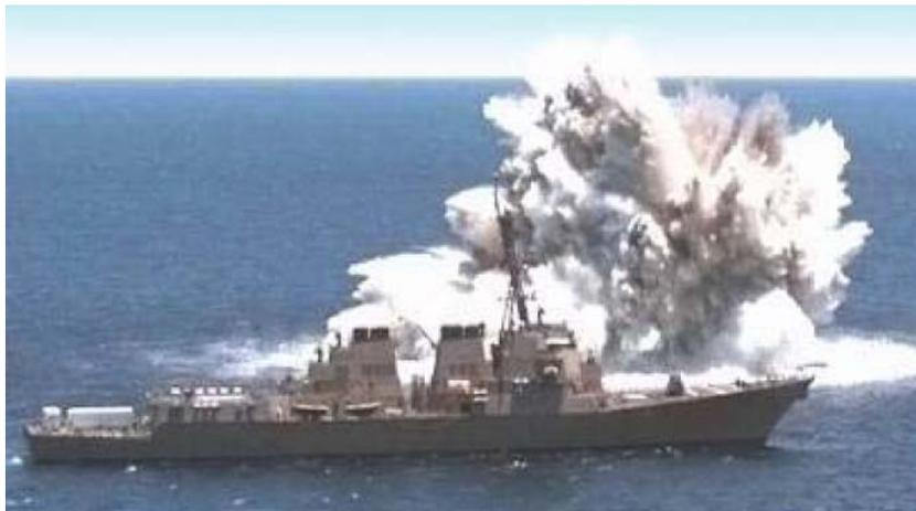
Figure 24: Full ship shock trial (FSST) (Sturtevant, 2007)
