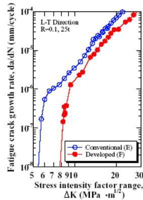
Figure 11: Fracture crack growth test results in atmospheric environment, Katsumoto *et al* (2005)
