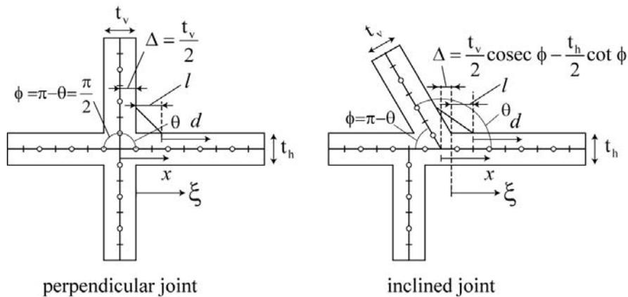
Figure 21: Distance of the read-out-points (ROPs) from the hot spot used in Osawa's method.
