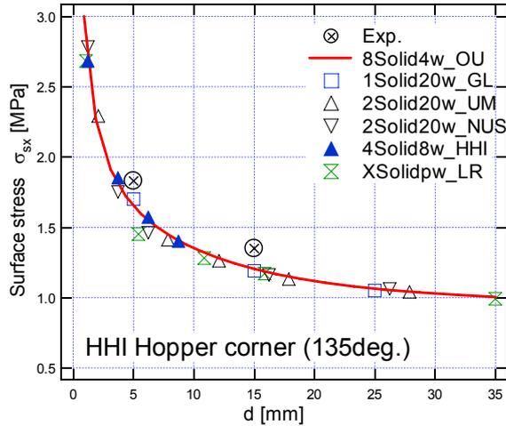
Figure 23: HHI Hopper corner (135deg.) model: comparison of solid surface stresses.
