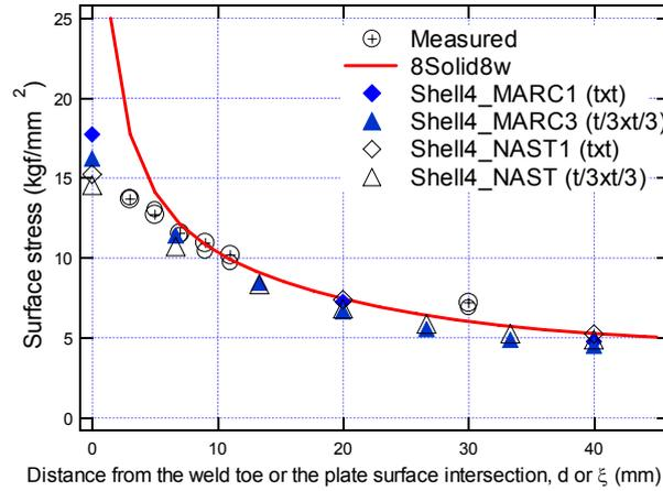
Figure 26: MHI right angle joint model: comparison of shell and solid surface stresses.
