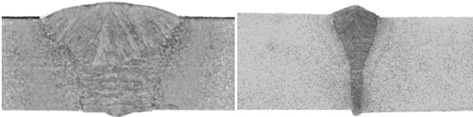
Figure 16: Difference between geometry of submerged arc (left) and laser hybrid (right) welded joint (Remes and Varsta, 2007).
