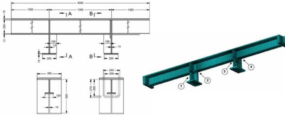
Figure 18: Structural details of the longitudinal / bulkhead penetration and typical finite element (Fricke *et al*, 2007a)
