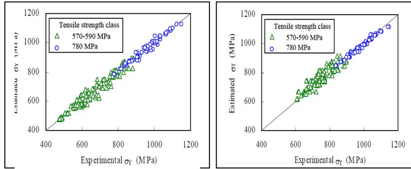
Figure 9: Comparison of estimated and experimental dynamic strength of pre-stained steel, Kuzbo *et al* (2007)
