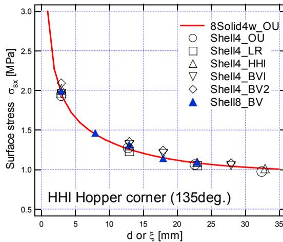
Figure 24 : HHI hopper corner (135deg.) model: comparison of shell and solid surface stresses.
