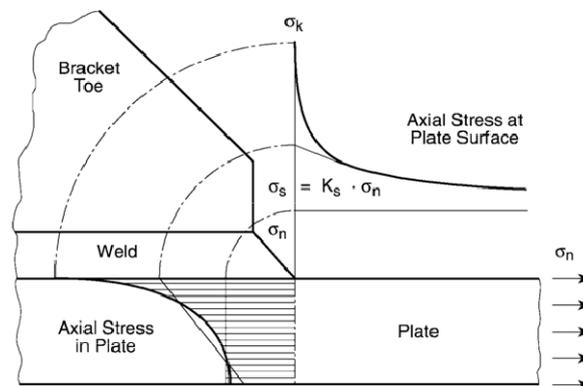
Figure 2: Stress types at a typical hot spot of a plate-type structure (Fricke *et al*, 2007a)
