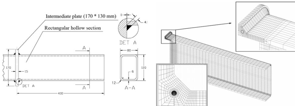
Figure 4: Test specimen geometry and a typical FE model (Fricke *et al*, 2007a)
