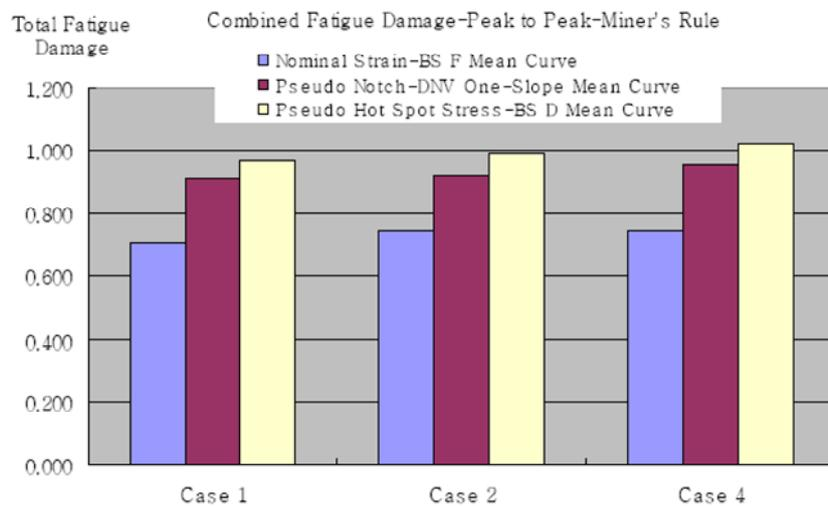
Figure 20 : Comparison of total fatigue damage calculation methods (Heo *et al*, 2007)
