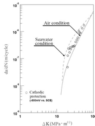
Figure 7: Corrosion fatigue characteristics of TMCP steel; see Kim and Paik (2007)
