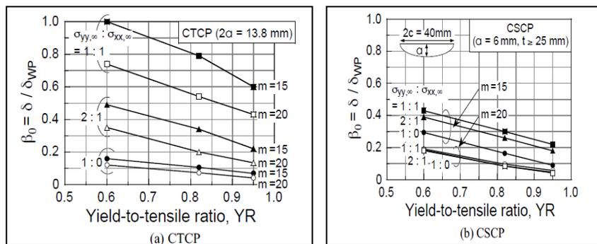
Figure 10: Effect of biaxial loading on the equivalent CTOD ratio  $\beta$  for CTCP and CSCP
