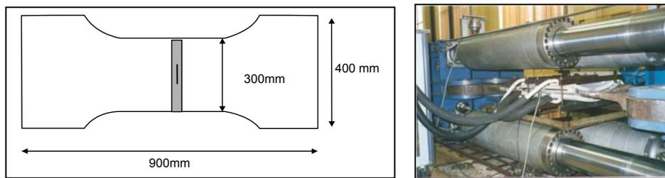
Figure 6: CWPT specimens geometry and test machine (Fairchild *et al* 2007)
