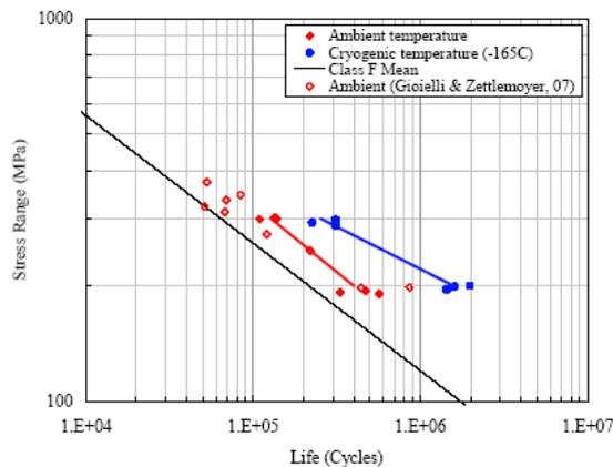
Figure 14: Fatigue test data of nine percent nickel steel at ambient temperature and cryogenic temperature (Gioielli and Zettlemoyer 2008)
