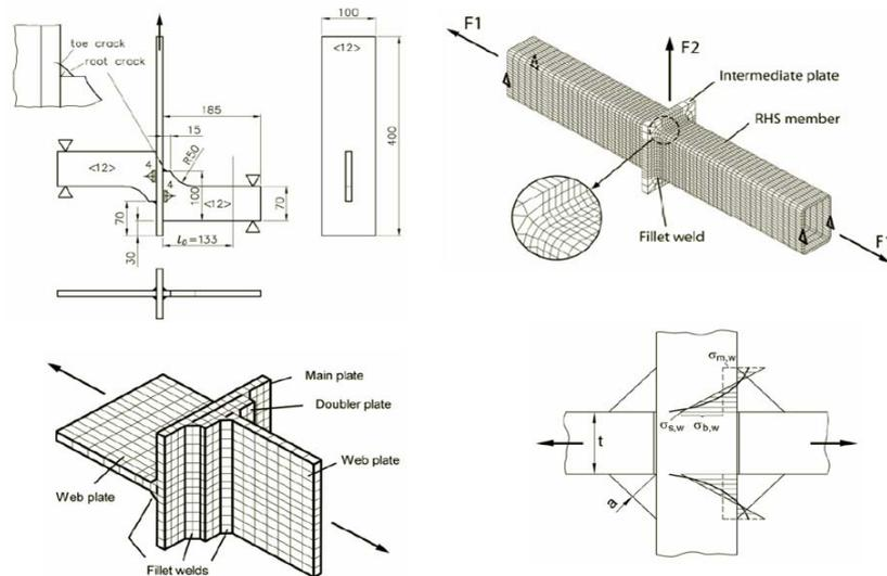
Figure 19: Examples of numerical and experimental study for weld root fatigue assessment (Fricke, 2006)
