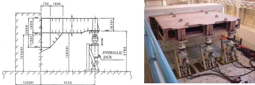
Figure 27: VLCC bilge knuckle model.
