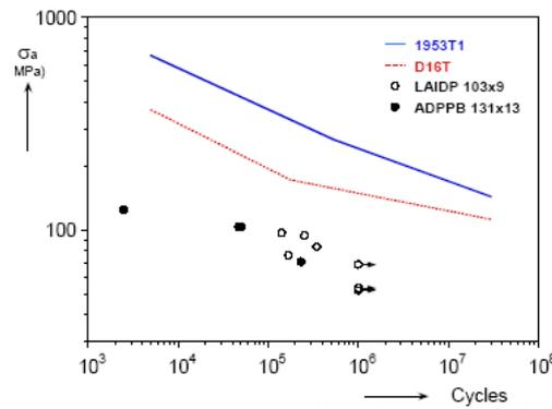
Figure 13: S-N curves based on small scale tests and full-scale results
