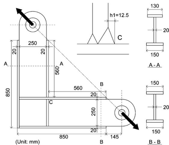
Figure 25: MHI right angle joint model.
