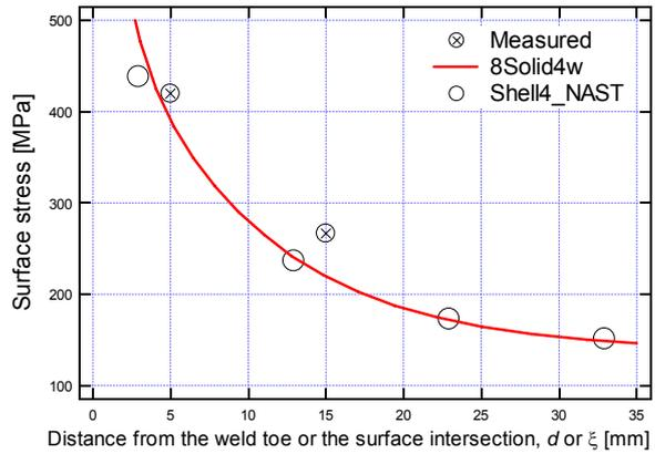
Figure 28: VLCC bilge knuckle model: comparison of shell and solid surface stresses.
