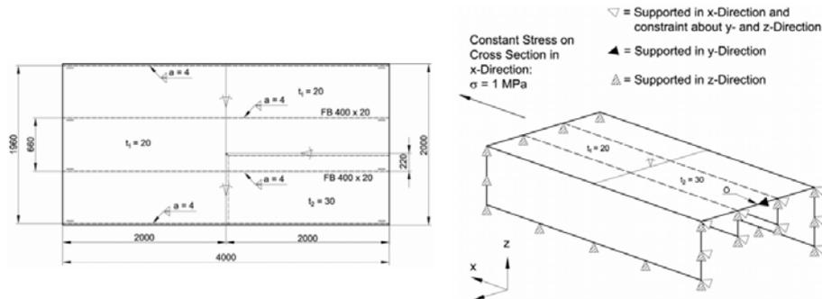
Figure 17: Geometry, boundary conditions and loads of deck strip with a thickness step (Fricke *et al* 2007a)
