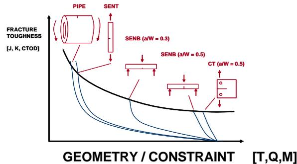
Figure 5: Fracture toughness compared by the constraint level for different specimens, Nyhus *et al* (2001).
