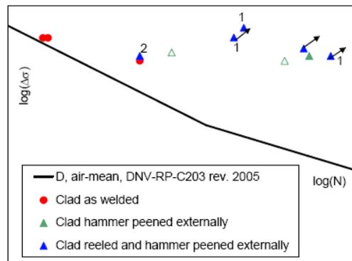
Figure 15: Nominal stress vs fatigue life for the different test parameters (Open symbols represents failure in pipe body.) 1) One specimen run-out tested at different stress levels. 2) specimen treated with partly fractured hammerhead, Kristoffersen *et al* (2008).
