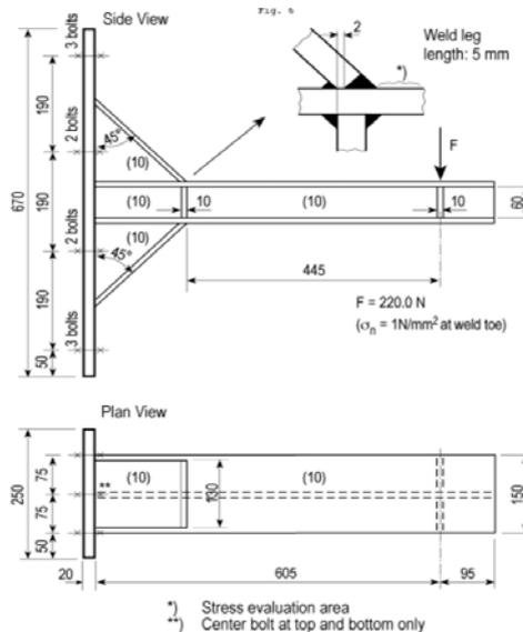
Figure 22: HHI Hopper corner model (135deg.).
