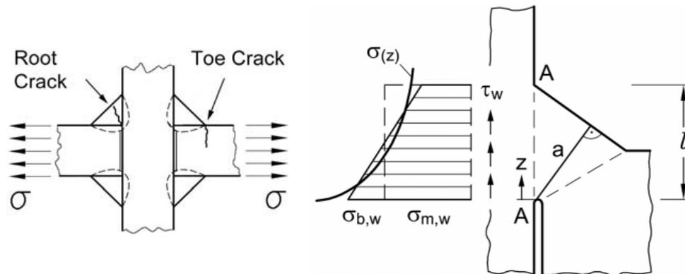
Figure 3: Possible fatigue cracks in fillet-welded cruciform joints and the linearization of stresses in the leg section of a partial-penetration fillet weld (Fricke, 2006a)
