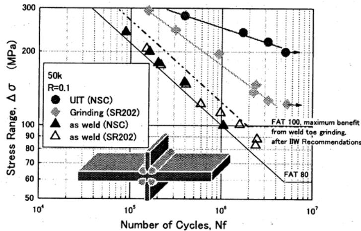
Figure 5: Effect of UIT on fatigue life in cruciform welded joint (Nose *et al.* 2007)
