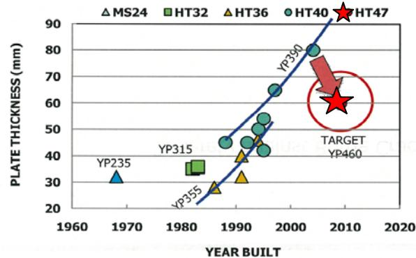
Figure 7: Specified yield point and plate thickness around hatch side coaming
