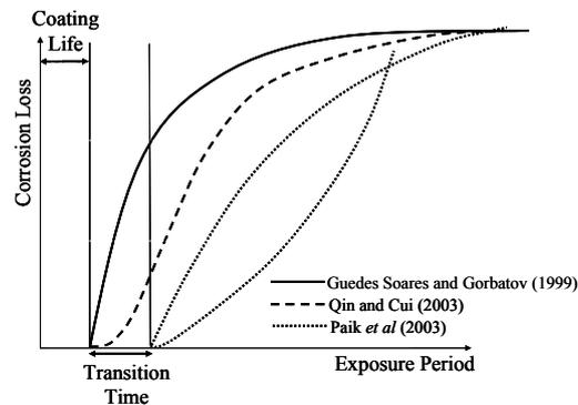
Figure 11: Schematic representation of models due to Guedes Soares and Gorbatov (1999), Paik *et al* (2003) and Qin and Cui (2003)
