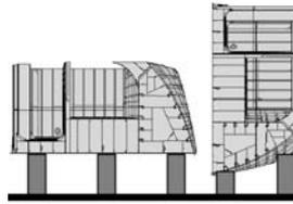
Figure 13: Application of bottom-up approach comparing shell-base production (left) and deckbase production approach (right); analysis gave 3% cost advantage for deck-base approach
