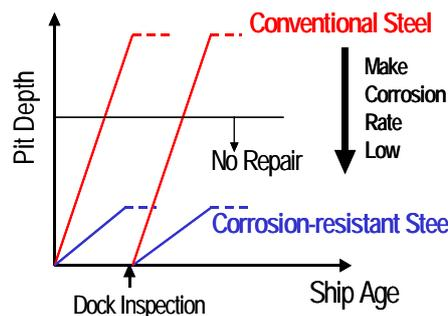
Figure 8: Repair free schematics for COTs built with corrosion-resistant steel
