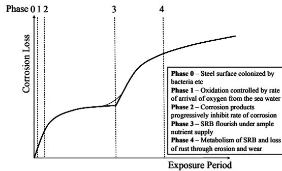
Figure 10: Corrosion loss model for immersion corrosion of steel in natural sea water (Melchers, 2007A)
