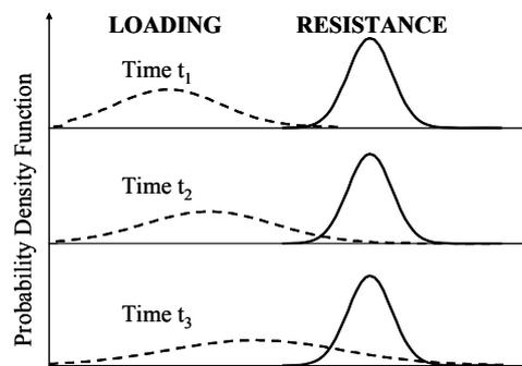
Figure 9: Effect of corrosion rate model in reliability assessments
